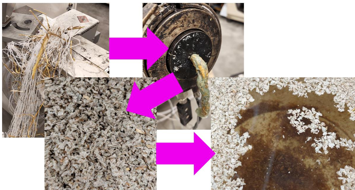
Figure 14. Straw bale netting compacting process and the final crushed material. Minimal mixing during the compacting process allows the straw particles to separate from the plastic.
