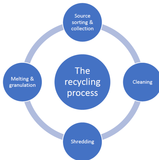
Figure 1. The mechanical recycling process of L-LDPE haybale wraps
