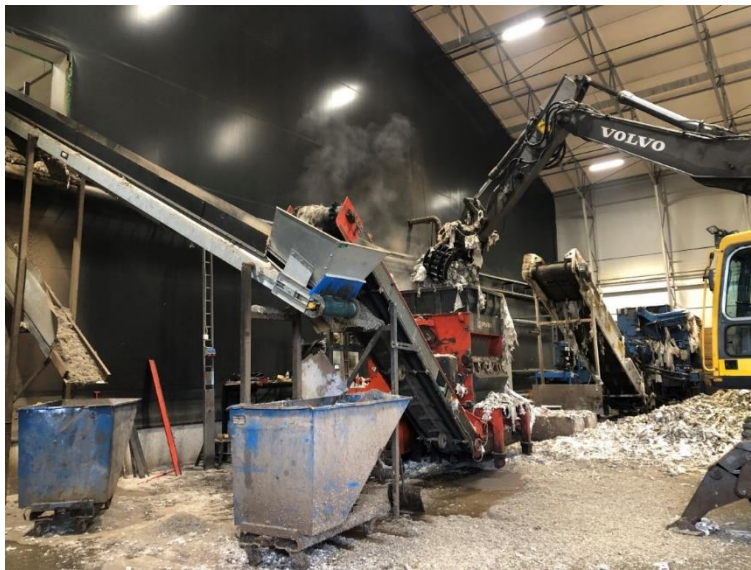
Figure 12. Crushed agricultural plastic waste fed to the granulation process (Veijo Pönni, 2024)
