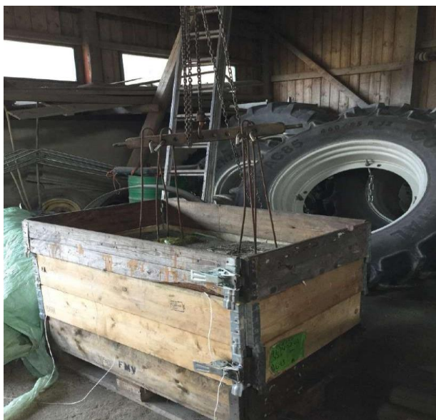
Figure 18. Self-made press to package bale wrap plastic waste. (Leena Erälinna, 2019)
