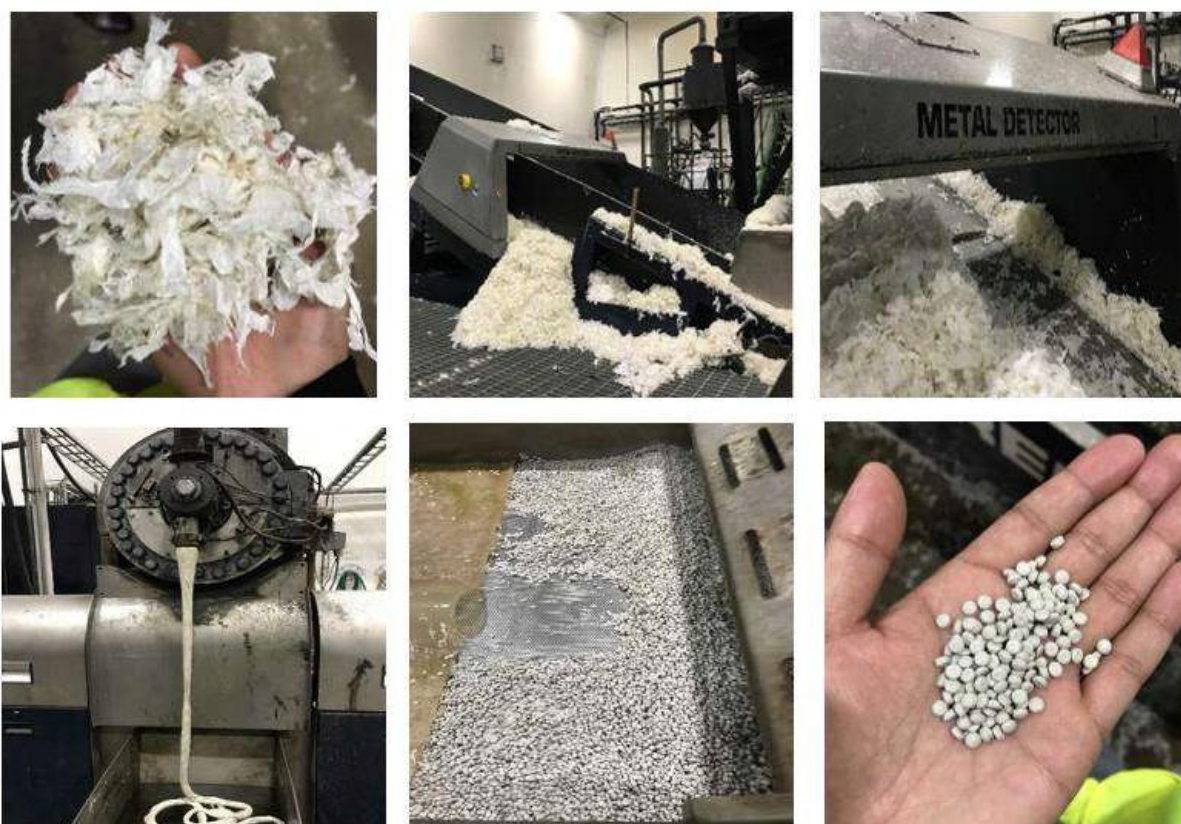
Figure 4. Recycling process of haybale wraps at Clean Plastic Finland (Aaqib Mohammad, 2024)
