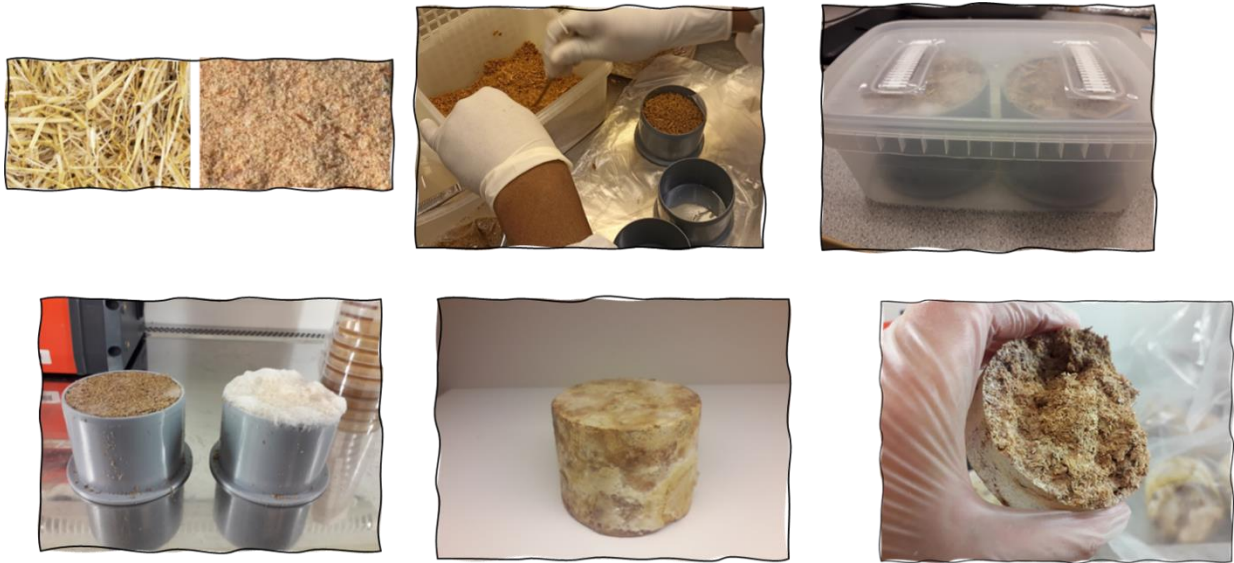
Fig 9. General steps for the production of mycelial composite materials. Photographs by Marta Cortina-Escribano
